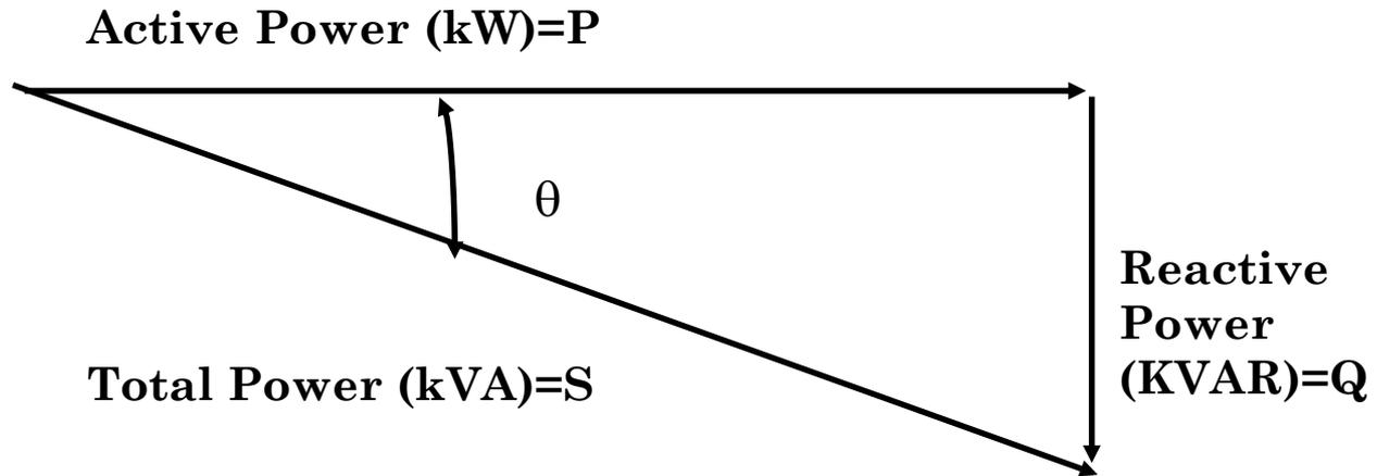
$$\begin{aligned}\text{Power Factor} &= \frac{\text{Active (Real) Power}}{\text{Total Power}} \\ &= \frac{P \text{ (kW)}}{S \text{ (kVA)}} \\ &= \text{Cosine } (\theta)\end{aligned}$$
