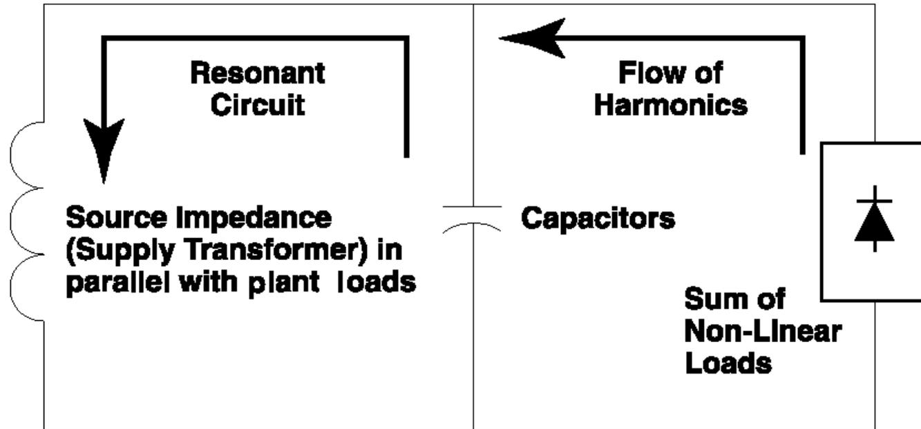
*The installation of standard capacitors can magnify harmonic currents on the network*
