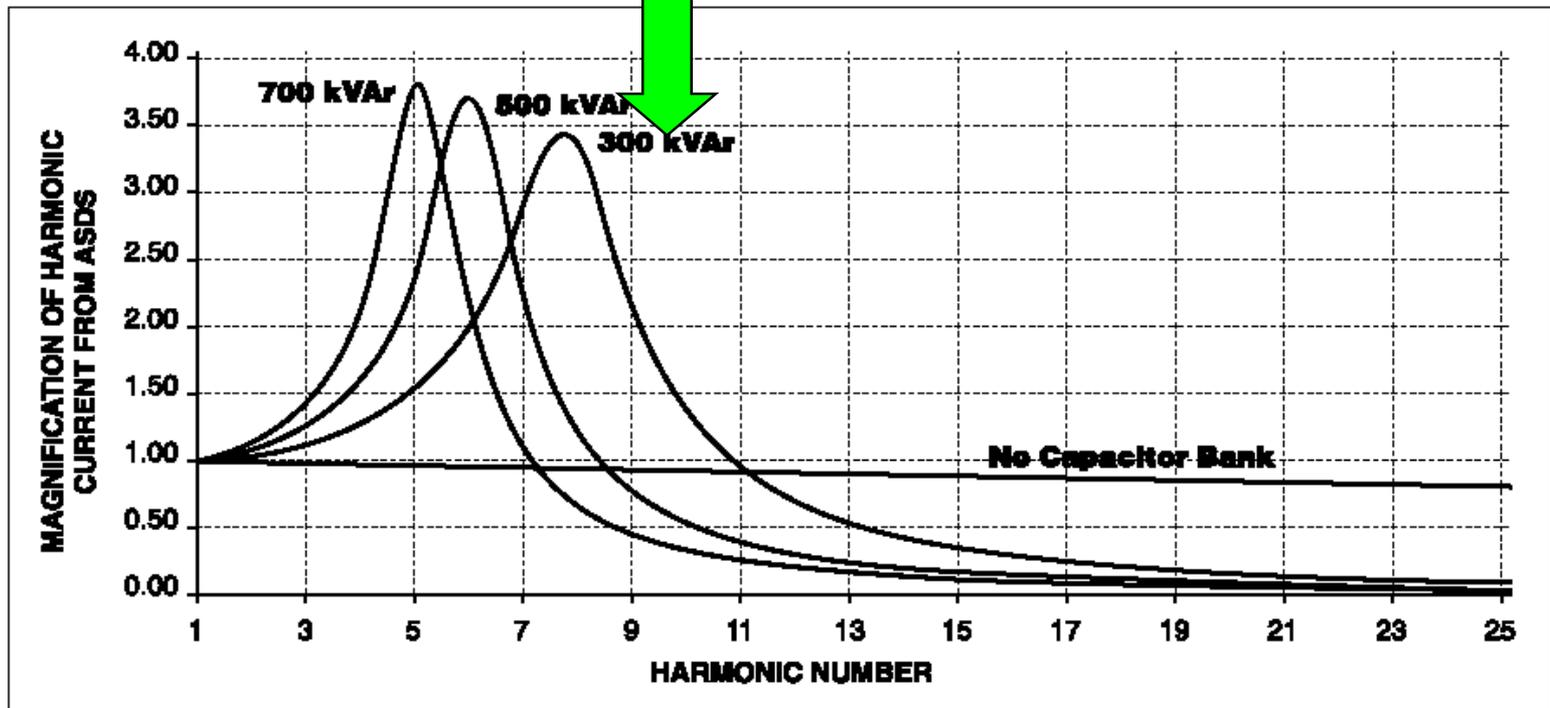
Magnification of Harmonic Current when Standard Capacitor are Added to the Network
