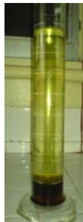
Figure 8 Products from 1-step transesterification of coconut oil
