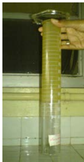
Figure 11 Solidified oil due to high FFA content
