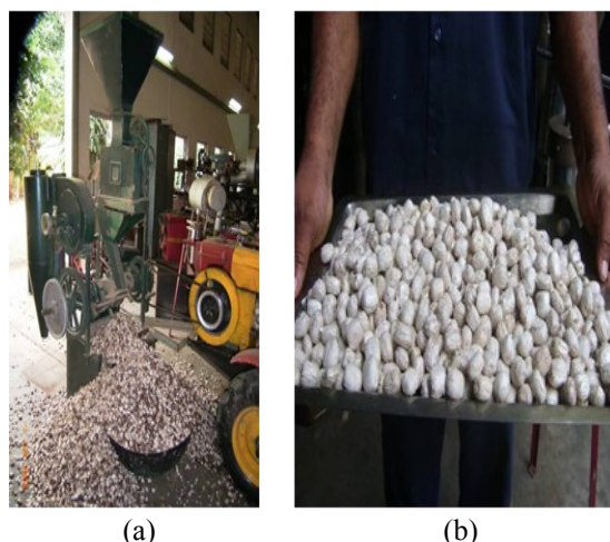
Figure 1 Dhulling of Rubber Seed (a) Huller, (b) Rubber seed kernel
