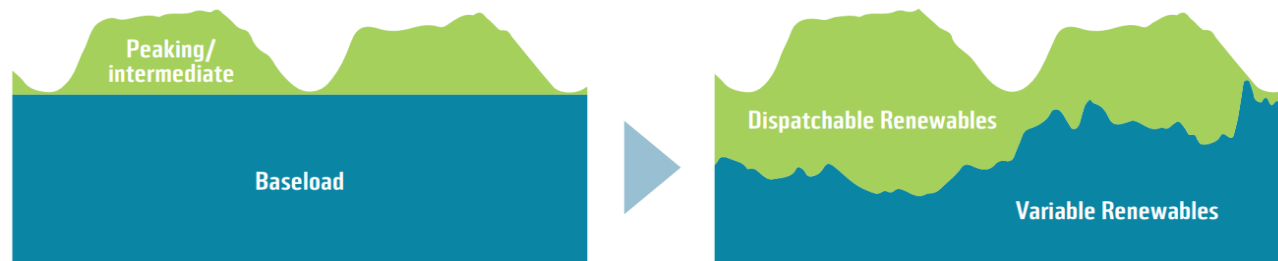
Figure 4: Transition from base-load to Renewables plus storage
