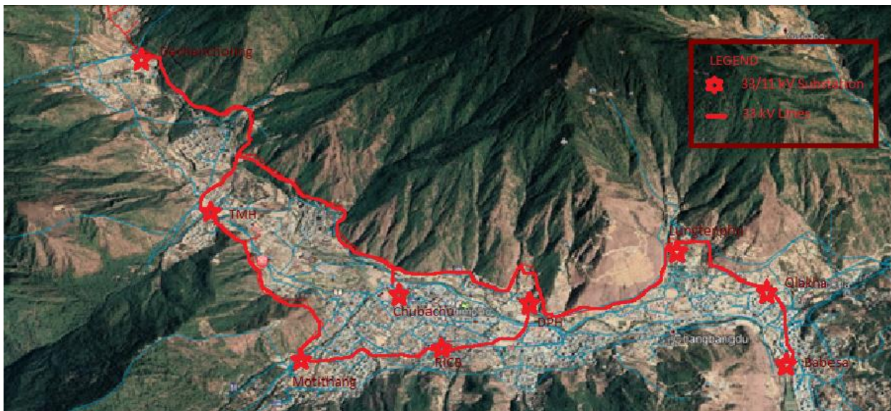
Figure 14: Overview of 33 kV Thimphu Distribution Network
