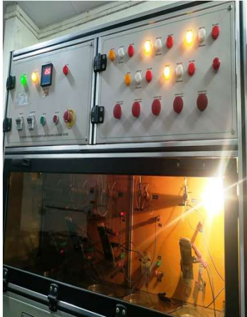
Track Resistance Test SetUP
