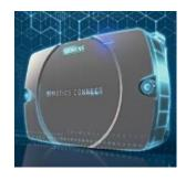
Sensors record temperature, vibrations, operating time, maybe also speed, torque
