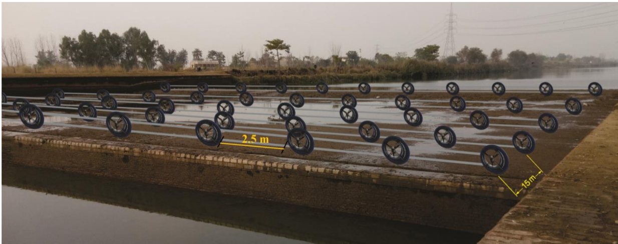
Figure 4-3: Proposed schematic arrays of the turbines that may be installed on one of the siphon head
