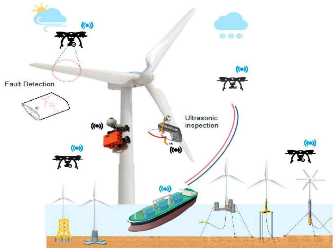
Fig. 8 Smart operation and maintenance technique [15].
