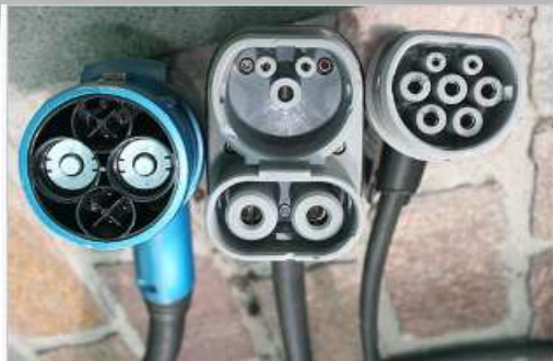
CHAdeMO connector (left), with the competing Combined Charging System (CCS) Combo 2 connector (middle), and the AC Type 2 connector (right)
