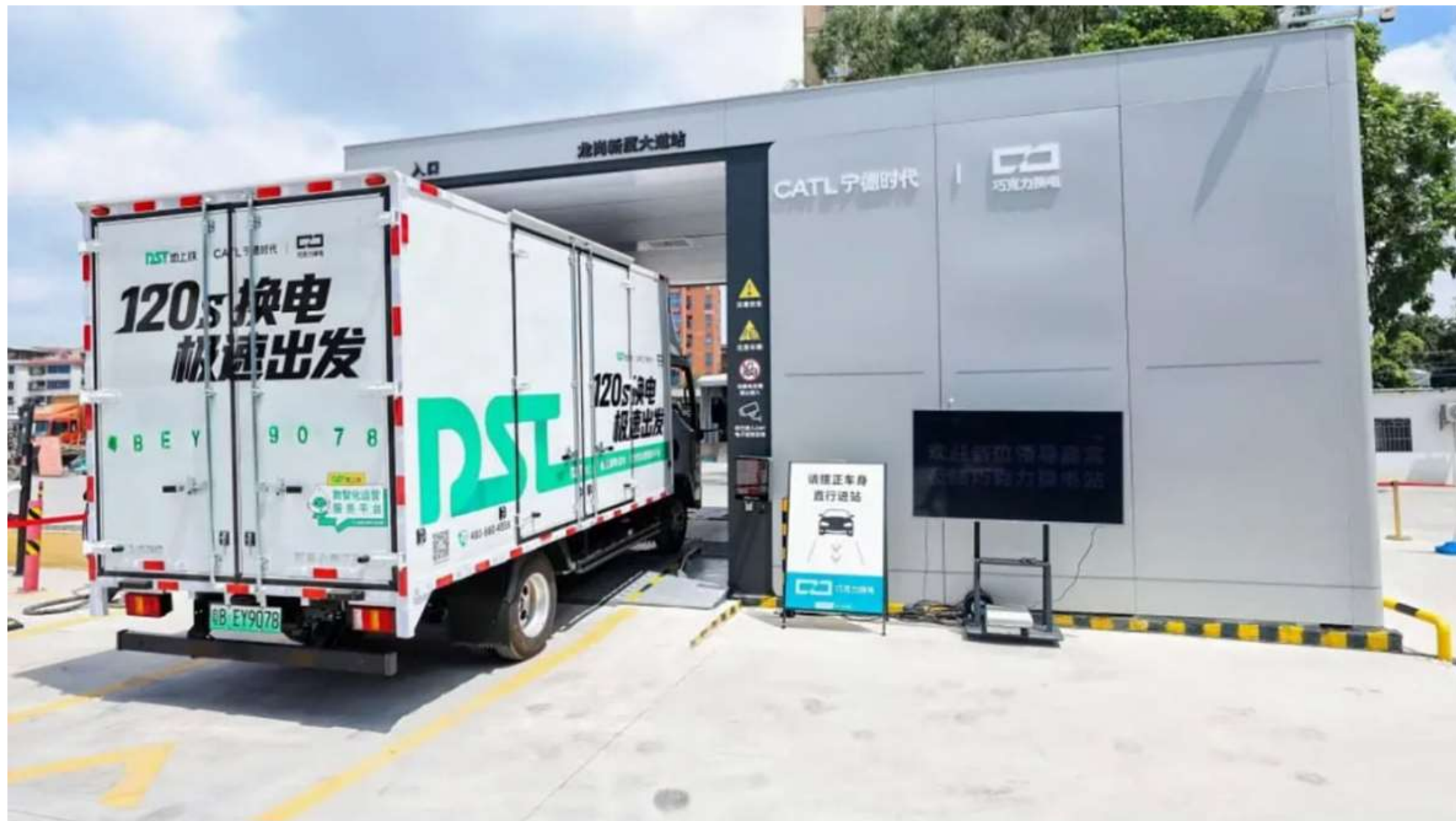
A light-duty truck undergoes battery replacement at a CATL battery swap station. Image credit: CATL
