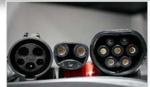
IEC Type 1/SAE J1772 inlet (left); NACS (center); IEC Type 2 connector outlet (right)
